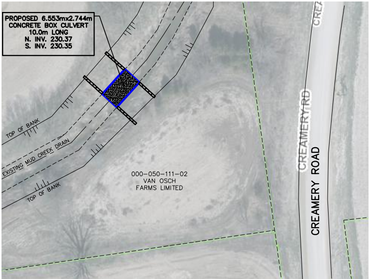
CONCRETE BOX CULVERT DETAIL PLAN NTS
