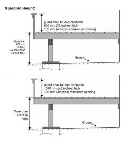
Figure 10: Example of Guardrail on Built-in Bench
