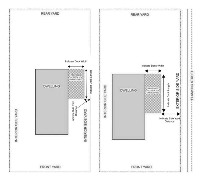
Figure 4: Example of Site Plan with Side Yard Deck
